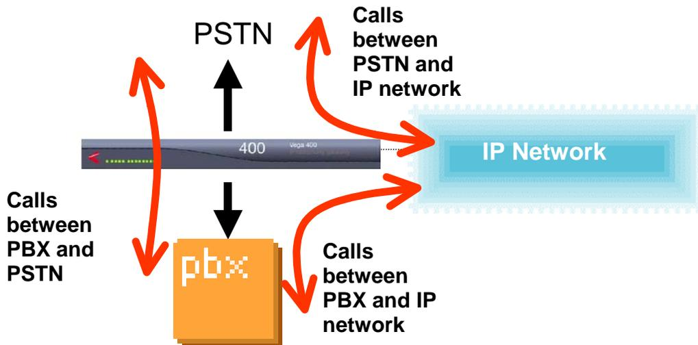
Because each of the Vega 400's four E1/T1 ports is independently configurable, it can simultaneously connect to both a PBX (NT mode) and the PSTN (TE mode), as well as the IP network. The Vega 400 has a uniquely powerful dial planner, enabling it to make call-routing decisions between each interface to minimise cost and maximise flexibility.
